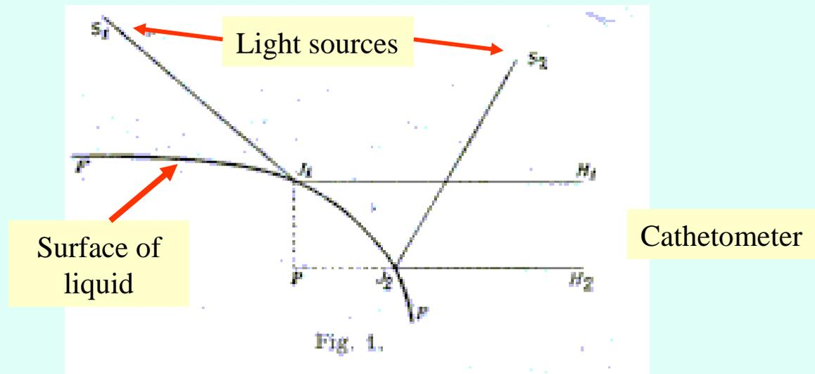
Reflection method of capillary measurements of Eötvös
