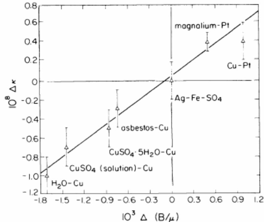
FIG. 1. Plot of  $\Delta \kappa$  vs  $\Delta(B/\mu)$  using the data in Table I.  $Ag-Fe-SO_4$  refers to the reactants before and after the chemical reaction described by Eq. (7). The solid line represents the results of a least-squares fit to the data.
