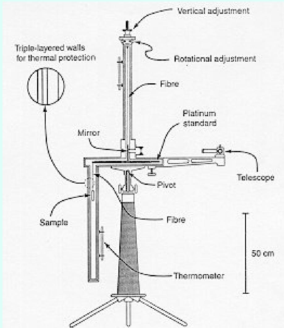
Eötvös-balance as used for UFF tests
