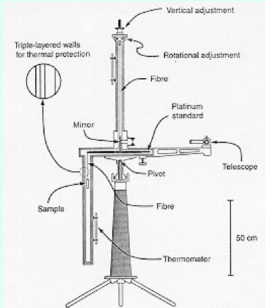
Eötvös-balance as used for UFF tests
