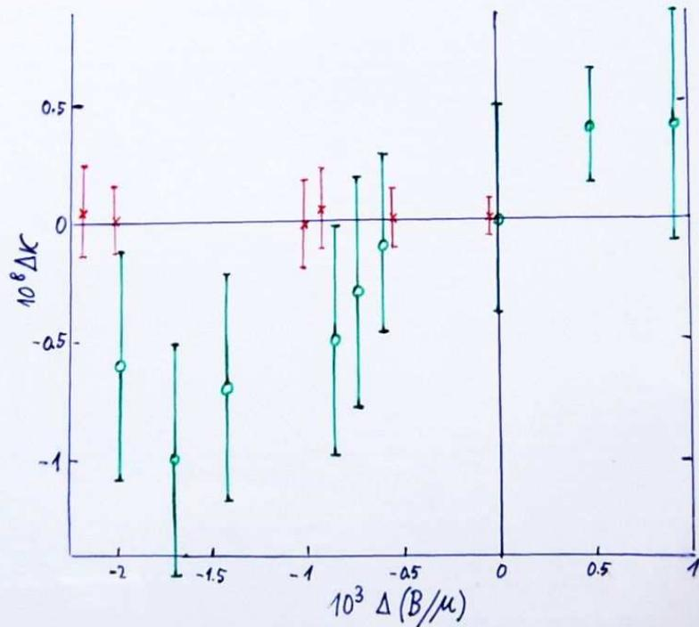
Differential accelerations measured by Eötvös, Pekár and Fekete (EPF) and by Renner (1930-35). standard deviations are 2.4 times larger than given by the authors!
