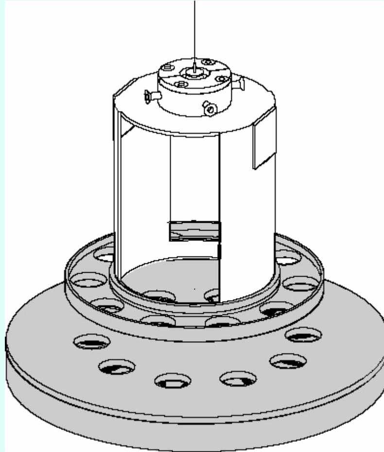
Most recent torsion balance of the „Eöt-Wash” group that checked the validity of the  $1/r^2$  law of gravitational attraction down to about 50 micrometers.
